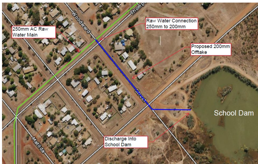
Figure 4: Raw Water Offtake to School Dam
