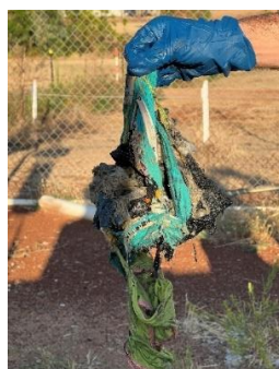
Figure 4 - Cause of Sewerage Pump Station 2 Fault on 04/09/23
